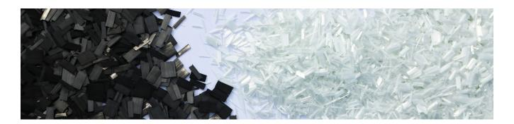
Xenia, specialised in the development and production of thermoplastic composites has recently introduced a new family of materials reinforced with hybrid fillers composed of carbon and glass fibres mixtures.
